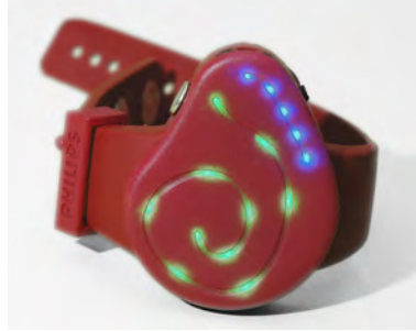
Figure 7.1: The Vitality Bracelet with all (green) lights for paced breathing on as well as all (blue) lights indicating the duration.
